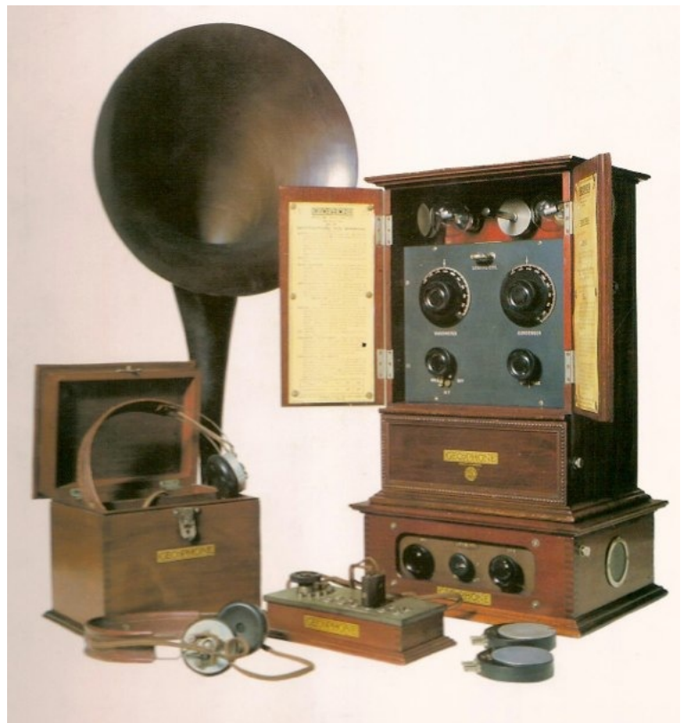
Fig. 132: Gecophone Smokers cabinet with speaker, headphones, coils and a headphone splitter which allowed several people to listen in via headphones. Picture Source Radio Art (Hawes, 1990)
