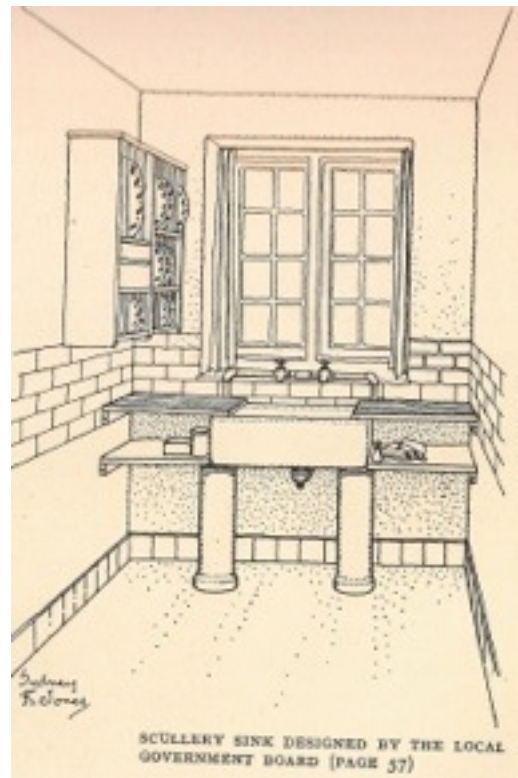
Fig. 115: The Studio Yearbook 1919 : certain aesthetic improvements were not based upon decorative schemes of vernacular styles; note hot and cold running water in this standard scullery designed by the Local Government Board as a way of improving the access to hygiene for the masses.
