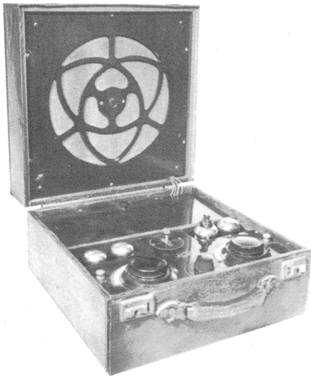
Fig. 123. Burndept “Screened Suitcase Portable” 1928 This model is atypical of the suitcase portables gained popularity during the late 1920s having evolved from an earlier portable type which did not fold away. Picture Source: Radio! Radio! (1996)
