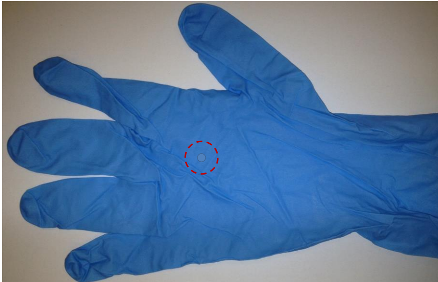
Figure 5.1. Mn sample dried for 30 minutes on a nitrile glove
