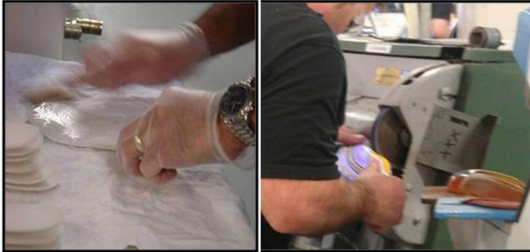
FIGURE 3.17: PRE-TREATMENTS OF (A) THE SLS SOLE UNIT WITH SATREAT 300 AND (B) ROUGHING OF THE INFERIOR SURFACE OF THE UPPER.
