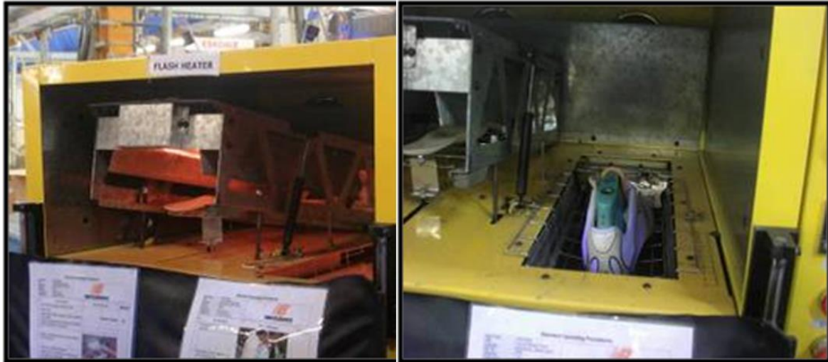
FIGURE 3.18: FLASH HEATER USED FOR THE ACTIVATION OF THE ADHESIVE
