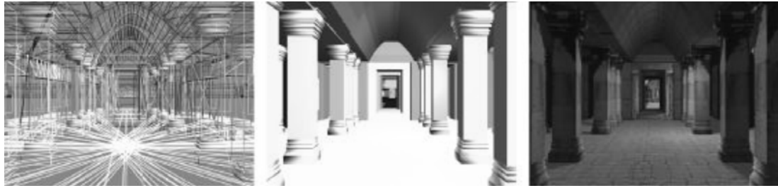
Figure 5-12 Interior perspective, wireframe, shaded, texture mapped view of the computer reconstruction of the central sanctuary, Phimai (R. M. Levy 2001)
