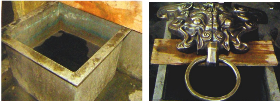
Figure 4-36 Dipping method of chemical colouring
