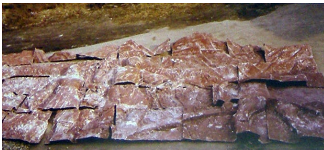
Figure 4-11 Drying glass-fibre sections in air
