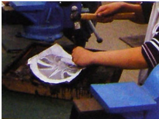
Figure 4-30 Chiselling the outlines
