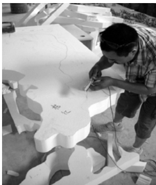
Figure 6-11 Cutting foam boards (left image)
