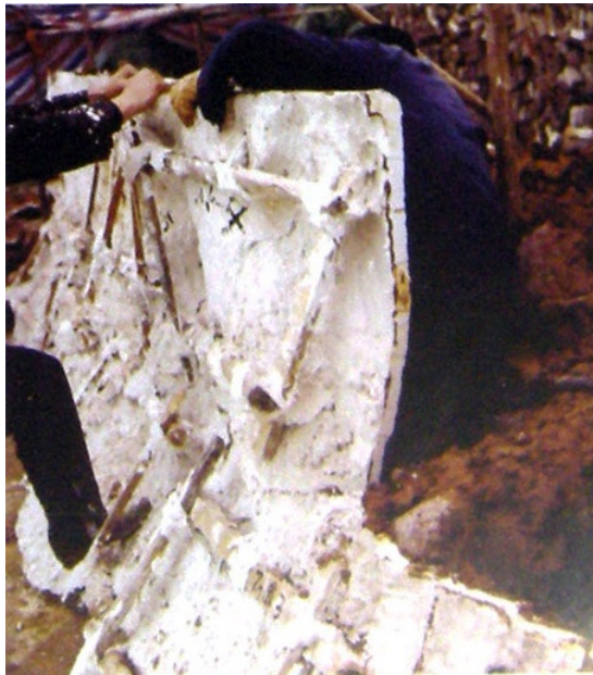
Figure 4-7 Disassembling the divisions and cleaning the clay off the inside (B. Lin, X. Chen, 2007)
