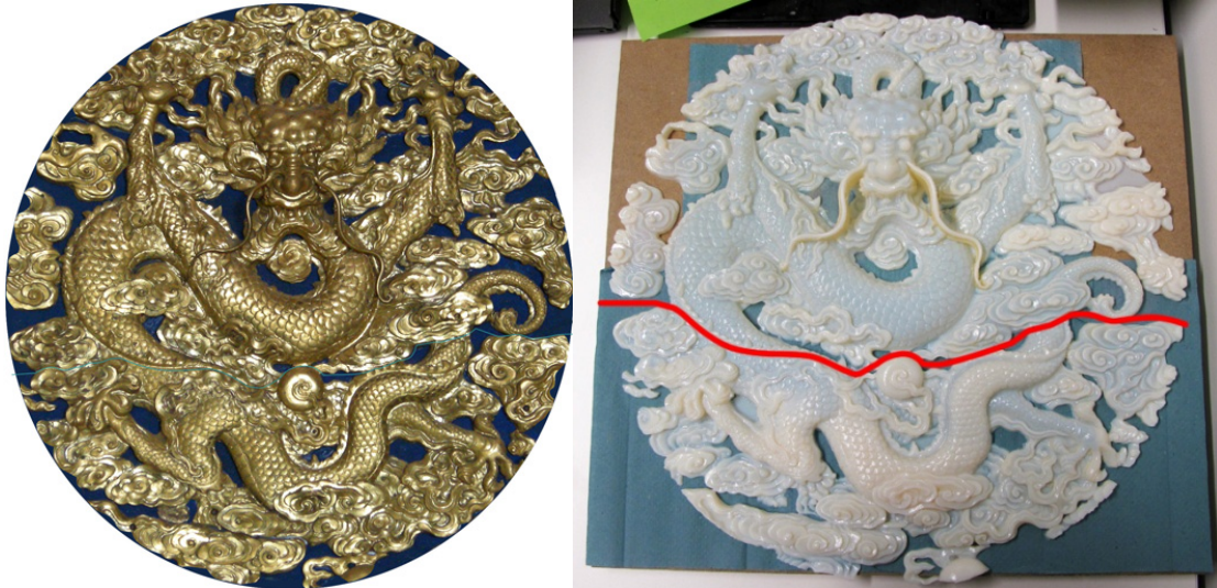
Figure 6-34 The chosen area from original artefact (left), the AM full size model with dividing line marked in red (right)
