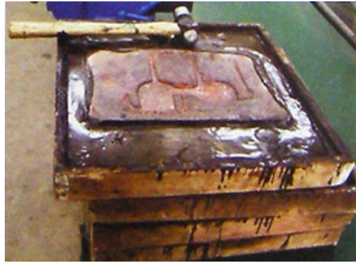
Figure 4-29 Bonding copper sheet to gluing platform
