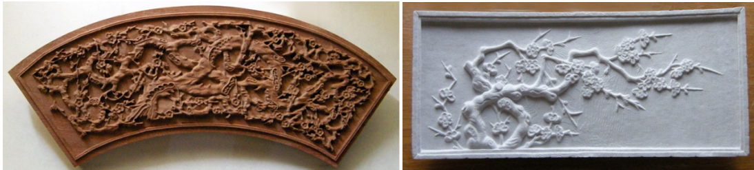
Figure 6-37 CNC wood ceiling part (left), coloured AM part simulating marble (right)
