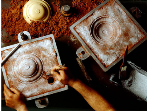
Figure 5-8 Mould holes & sprues
