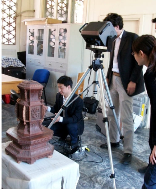
Figure 2-23 3D scanning process
