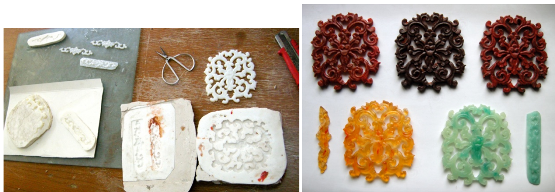
Figure 6-33 Rubber casting from AM parts (left), simulation of different materials (right)
