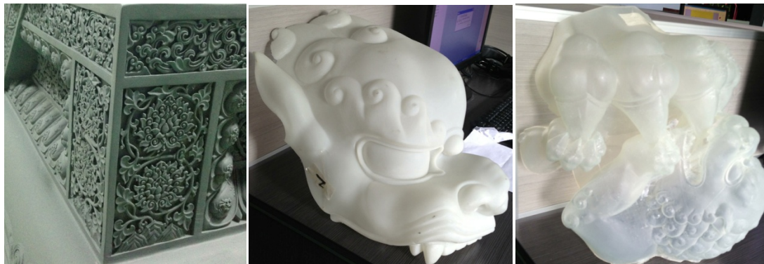
Figure 8-17 AM parts - relief with undercuts, lion's face, claws with baby lion
