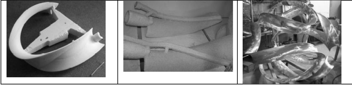
Figure 3-7 Plastic foam segment; Wax pattern with ceramic shell; Bronze model
