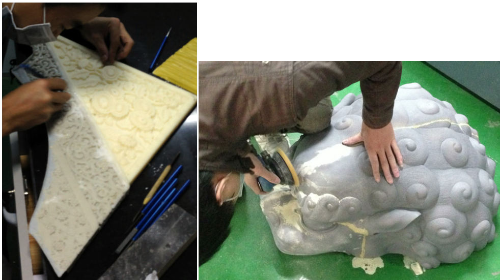
Figure 8-19 Removing support material manually and surface finishing
