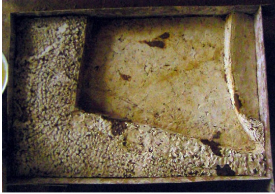
Figure 4-8 Female mould with enclosure
