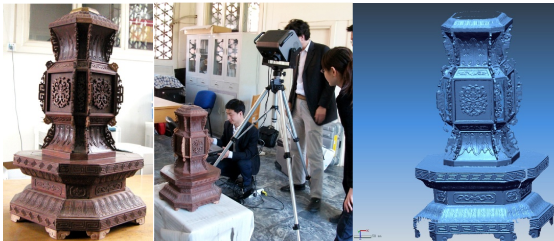
Figure 6-27 Original artefact (left), 3D scanning process (middle), the scanning data (right)
