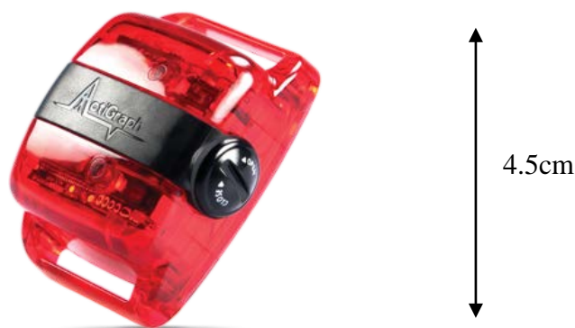
Figure 11. Image of GTX3+ accelerometer (Image from http://www.actigraphcorp.com/products/ )
