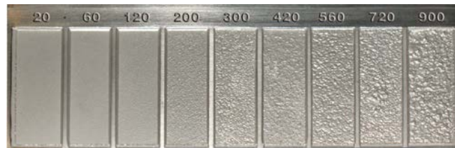
Figure 3.7: Micro-finish comparator (AFS, 2013)
