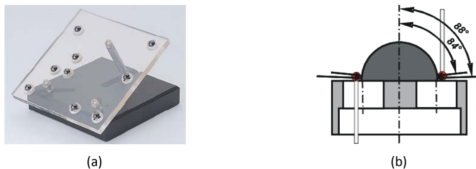
Figure 2.15: (a) Zeiss hemisphere plate; (b) two approach directions by tactile micro-probe (PTB, 2012)
