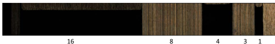
Figure 7.8: Line measurement of all staggered gauge blocks with the 2.5x lens
