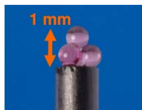
Figure 2.25: Micro-tetrahedron standard for CT scanners (Neuschaefer-Rube et al., 2013)
