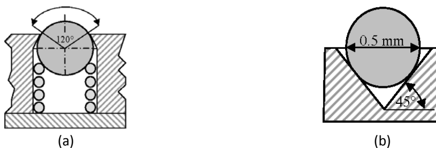
Figure 2.17: (a) Fixing principle with pressure springs; (b) adhesively bonded spheres (Ehrig and Neuschaefer-Rube, 2007)
