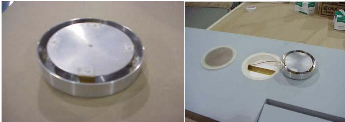
Figure 1:2: Embedded annular slot antenna integrated on to a wing structure (from Engle, R [6])
