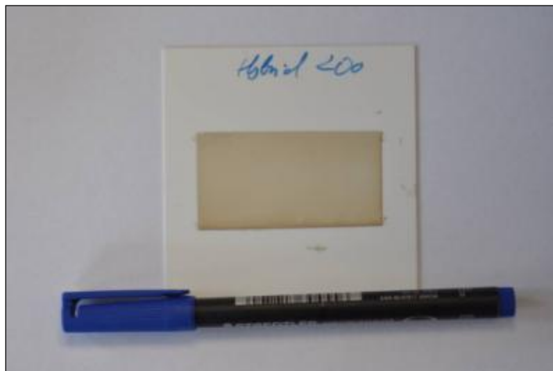
Figure 6:1: DW Silver hybrid ink sample applied to Alumina Tile for conductivity measurement.
