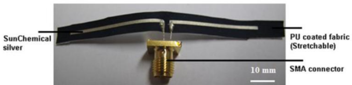
Inkjet printed 2.4 GHz dipole antenna on Plastibert (PU coated stretchable textile).
