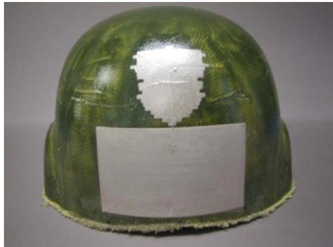
Broadband antenna and ground plane written on military helmet
