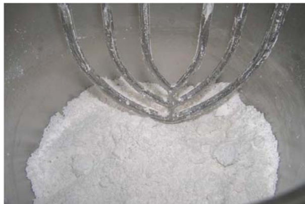
Figure D.6: Wet granules of Paracetamol.
