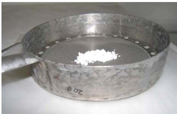
Figure D.7: Granules on #20 Mesh.
