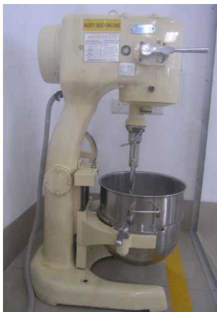
Figure 3.9: Mighty Mixer Granulator.
