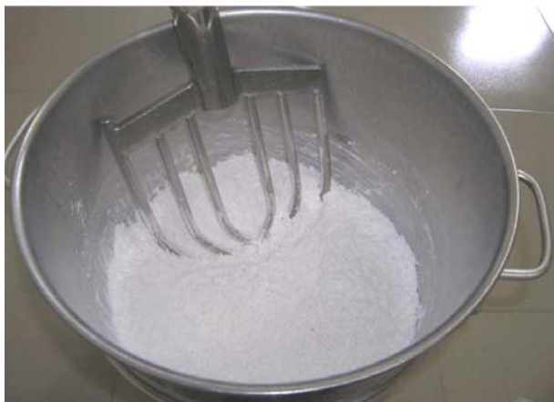
Figure D.5: Dry granules of Paracetamol.
