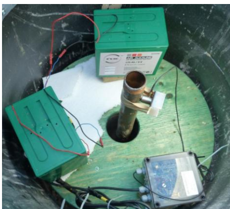
Figure 14. Waveguide with piezoelectric transducer attached, AE sensor, and batteries inside surface cover
