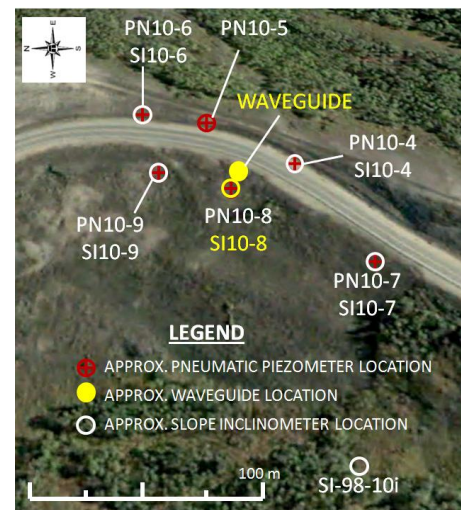
Figure 12. Instrumentation location plan at the Michelin slide, the location of the Slope ALARMS waveguide and the closest inclinometer (SI10-8) are shown in yellow
