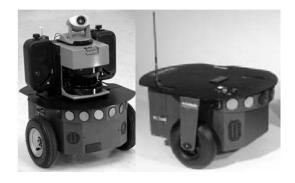
Figure 3.9: Pioneer-3DX mobile robots [44]
