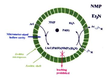
Figure 4.1 Schematic illustrations for the encaged quasi-homogeneous Heck-coupling in Pd@S1 catalyst.<sup>225</sup>
