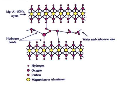
Figure 4.3 Structure of hydrotalcite.<sup>234</sup>
