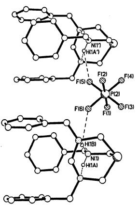
Figure 3.10 Molecular structure of 193 showing intermolecular H-bonding contacts between the  $[PF_6]^-$  counterion and cations.
