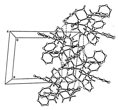
Figure 2.10 Packing plot for compound 169 showing N-H···Cl and C-H<sub>2</sub>···Cl interactions between molecules forming a chain parallel to a.
