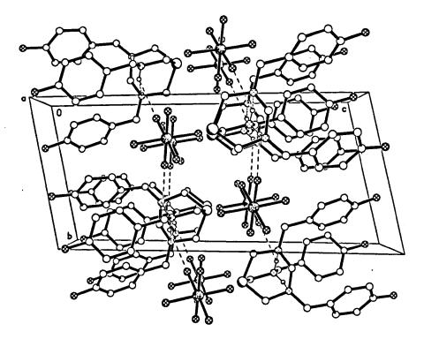
Figure 3.7 Packing plot for compound 190, parallel to *a* showing H-bonded chains of cations and anions.
