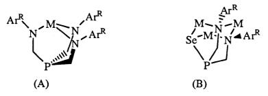
Figure 1.8 Potential bonding modes of the formally trianionic ligands  $P(CH_2NAr^R)_3$  and Se= $P(CH_2NAr^R)_2$  to form metal complexes.<sup>59</sup>
