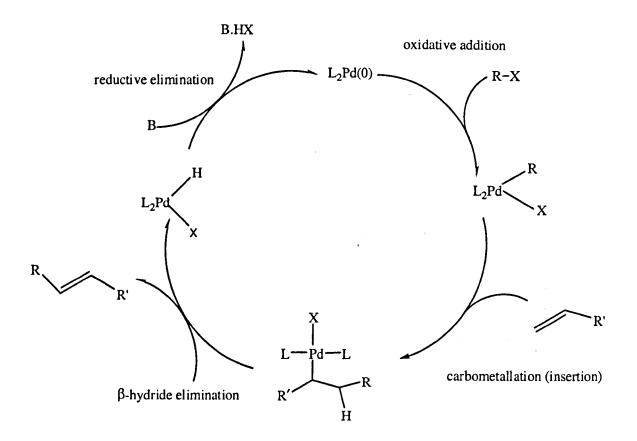
Figure 4.2 The Heck cycle (R' = electron-withdrawing group).
