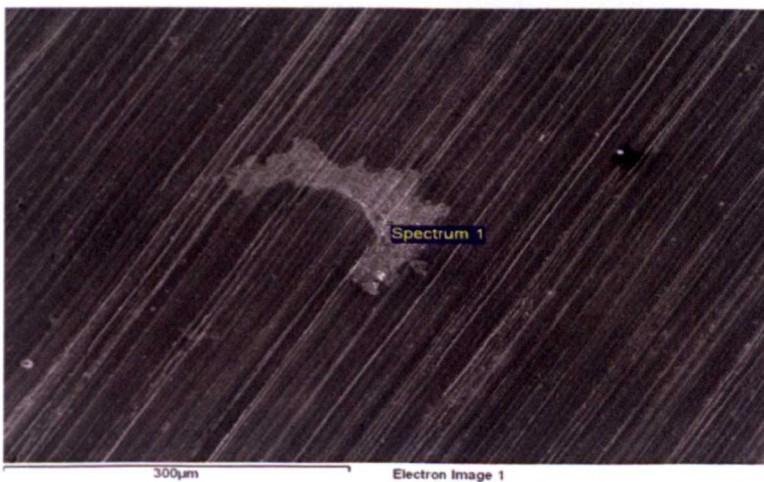
Fig 7-3: SEM image of plasma treated surgical forceps.
