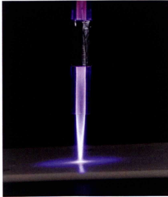
Fig 4-9: Digital image of a pulsed argon APGD Jet
