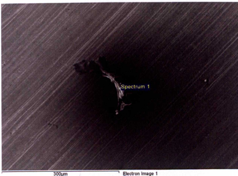
Fig 7-1: SEM image of contaminant on surgical forceps after traditional decontamination procedure.
