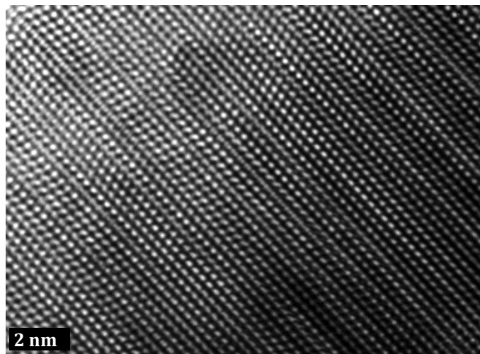
Fig. 2. A high-resolution TEM image of a CdTe grain from an untreated cell showing a high density of extended defects
