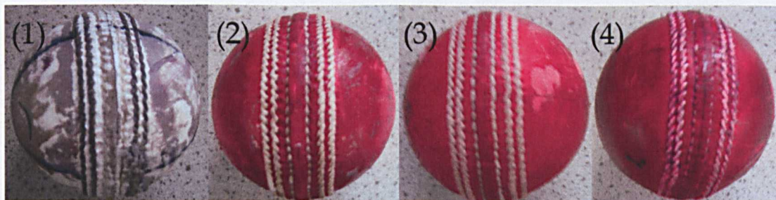
Figure 7.2.6: The four balls used during testing; 1: A white worn Readers, 2: A red new Readers, 3: A red worn Readers and 4: A red worn Slazenger.
