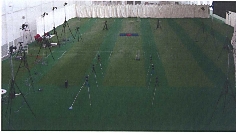
Figure 3.2.12: Extensive Vicon setup for player analysis.
