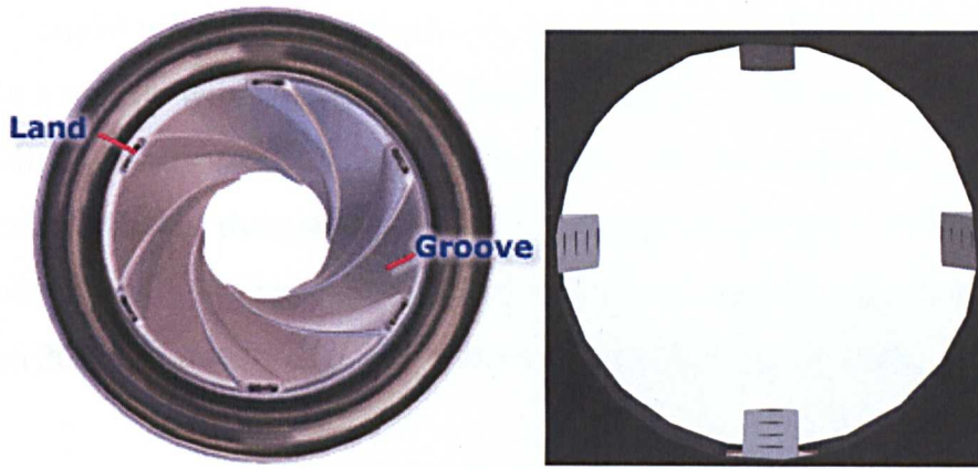
Figure 6.1.2: The rifling principle, as seen looking down a rifle barrel (left) (Doyle, 2005 - www.firearmsid.com ) and the rifling principle adapted for the spin head design, as looking down the machine barrel, right.
