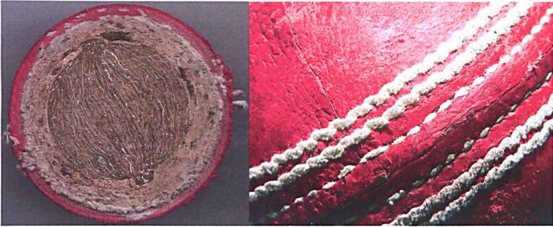
Figure 2.2.1: The internal construction of a cricket ball (left) and the protruding seam of the cricket ball (right) (Eager, 2006).
