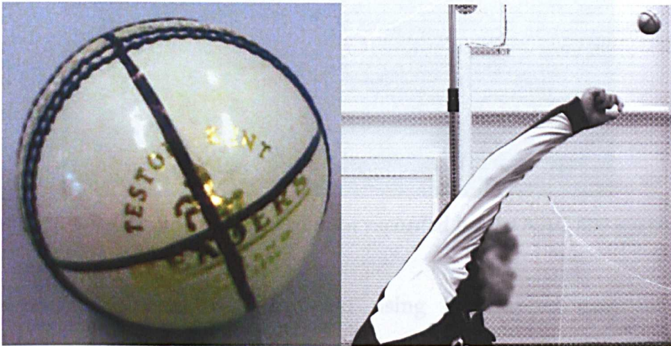
Figure 3.3.4: The markings placed upon cricket balls prior to testing (left) and a ball during testing (right).
