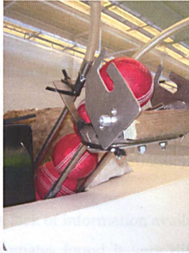
Figure 2.6.7: Merlyn's ball feeding device.
