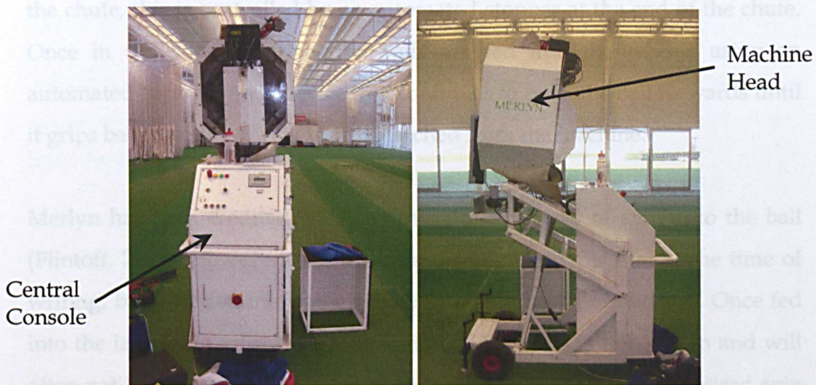
Figure 2.6.6: The Merlyn bowling machine.
