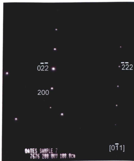
Figure 6.25 MAR M509 20,000 hours 950°C sample (a) FIB SEM image sample position (b) TEM image of thin foil and (c) diffraction pattern.
