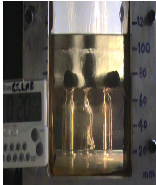
Figure 5-29: (b) Vigorous bubbling within the fuel layer in which the heater assembly was located was observed after 1200 s of heating
