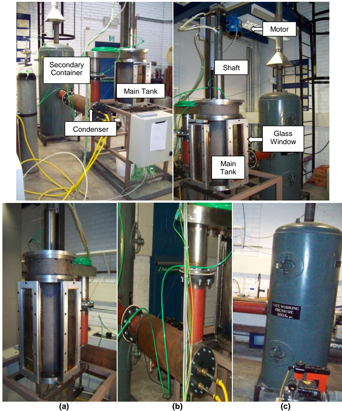
Figure 4-4: Boilover Experimental Rig: (a) Main Tank, (b) Condenser & (c) Secondary Expansion Container
