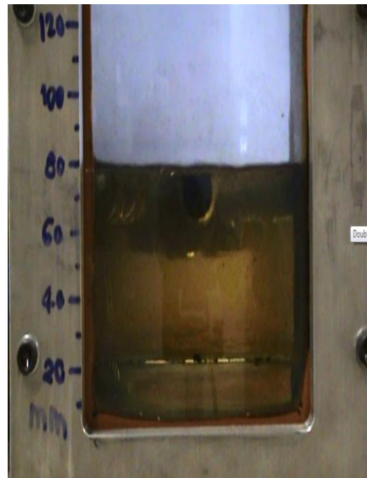
Figure 5-12: Photo of Laboratory Boilover Test LS Test 13 involving gasoline (b) After 420 s of heating – surface level is approximately at 80 mm from tank base
