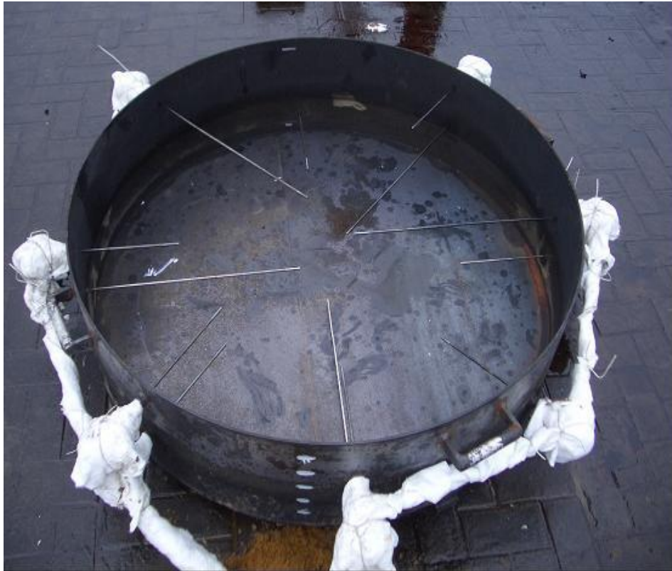
Figure 3-2: (a) Photo of thermocouples placement in the 1.2 m diameter tank
