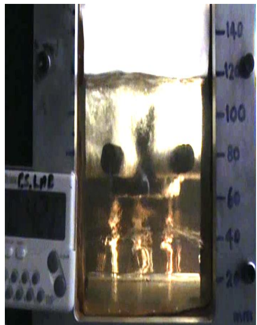
Figure 5-29: (d) Isothermal layer penetrated thin layer of fuel just below the heater assembly at 2520 s after heating
