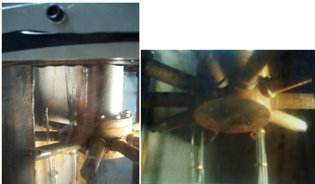
Figure 4-6: Cartridge heater assembly with ten cartridge heater elements
