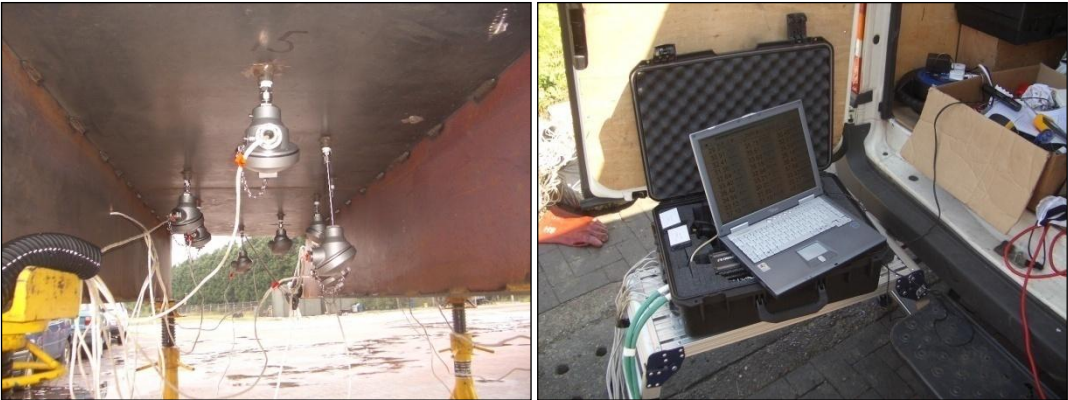
Figure 3-3: (b) Temperature probes connected to laptop / workstation in real time.
