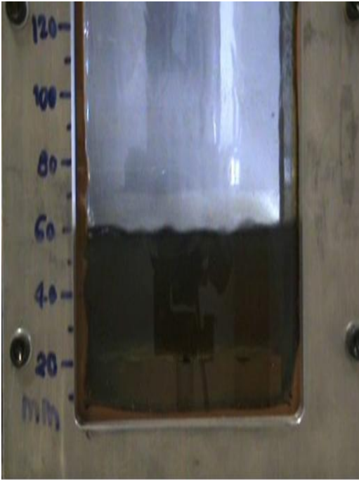
Figure 5-12: Photo of Laboratory Boilover Test LS Test 13 involving gasoline (c) After 900 s of heating – surface level is approximately at 60 mm from tank base
