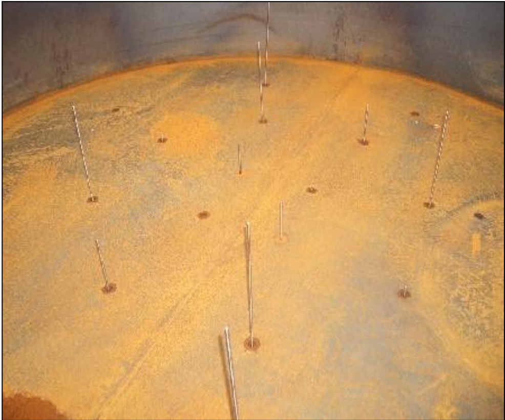
Figure 3-3: (a) Photo of the 2.44 m diameter test pan with thermocouples placement
