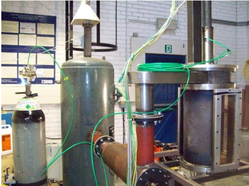
Figure 4-9: Nitrogen ( N_2 ) Gas System – N_2 cylinder is connected by the green tubing to the main tank
