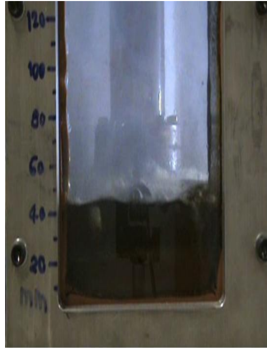
Figure 5-12: Photo of Laboratory Boilover Test LS Test 13 involving gasoline (d) At the end of the experiment – surface level has dropped to about 40 mm level mark. Vigorous boiling/bubbling did not occur.
