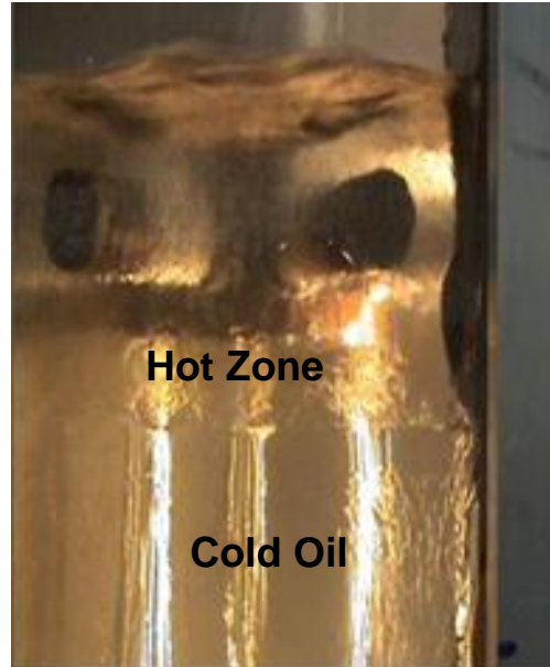
Figure 5-5: (b) Formation of hot zone: Hot zone started to be visible. Base of the hot zone regresses below the heater assembly after about 600s of heating
