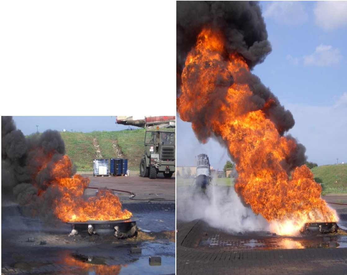
Figure 7-1: Photographs taken during progression of steady burning (left) and the boilover occurrence (right) of FS Test 5. Take note on the difference of the size (height) of the fireball-like flame during the occurrence of the boilover.
