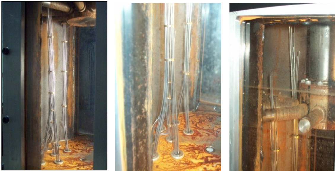
Figure 4-8: K-type thermocouples of 1.5 mm probe diameter placed at 10 mm height intervals from the tank base for detailed and fast measurements within the liquid
