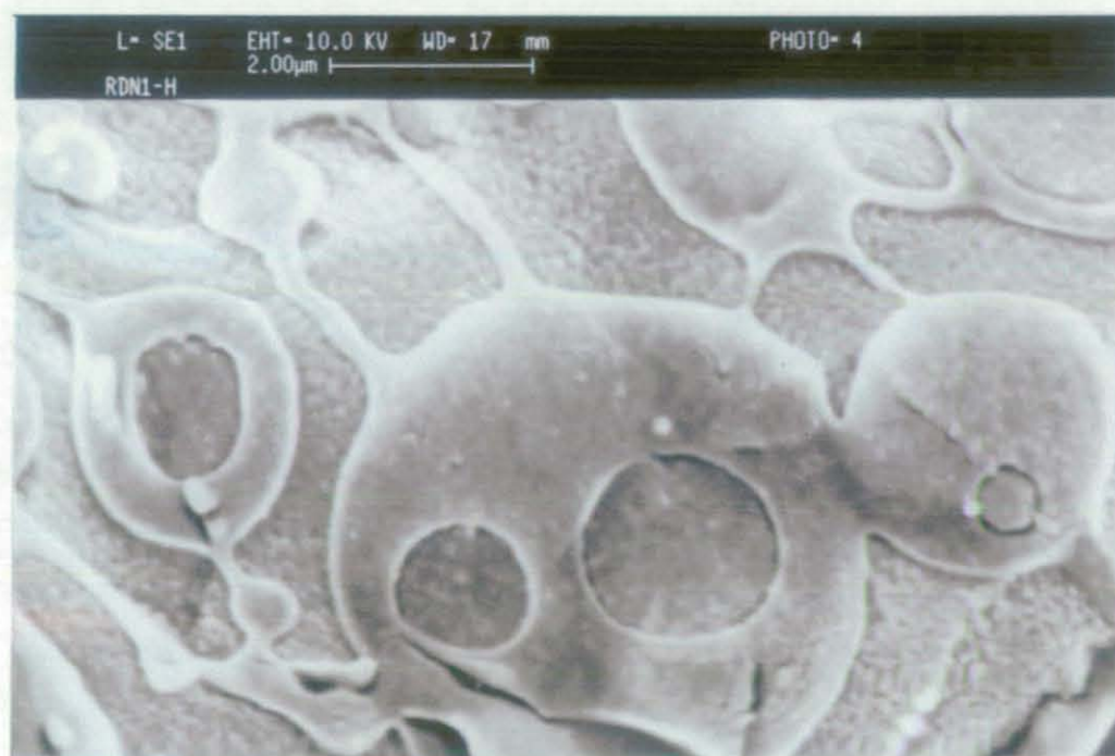
Figure 6.14c. SEM image of emulsions in the RIIW region: Showing the existence of small drops \sim 0.8 \mu\text{m}
