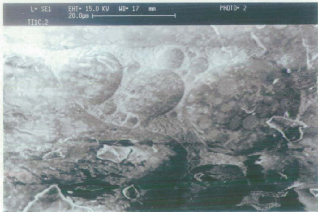
Figure 6.31. SEM image of RIITI experiment: Before complete transitional phase inversion
