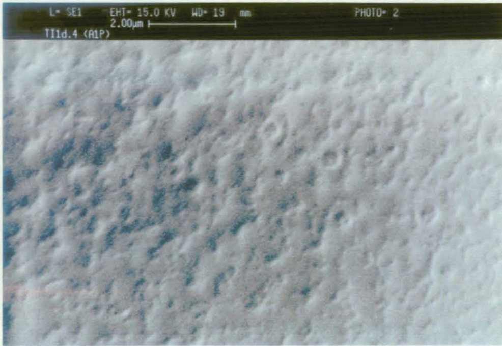
Figure 6.26. SEM image of RIITI experiment: Immediately after phase inversion
