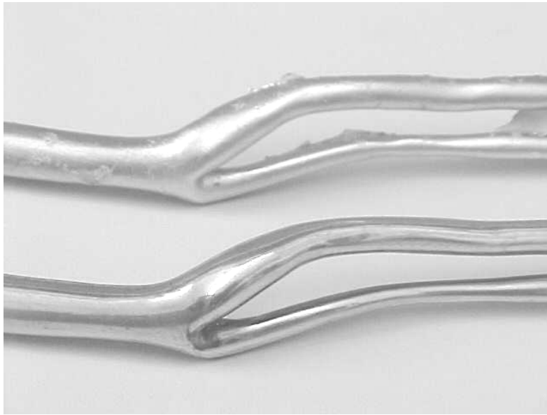
Figure 6: Low melting point expendable alloy cores for use in investment casting, as cast (top) and after hand finishing and polishing (bottom).
