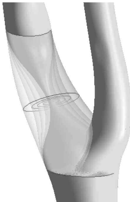
Figure 5: Manipulation of healthy CAD model to artificially simulate varying degrees of narrowing.
