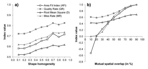
Fig. 12. Effects of changing (a) the shape homogeneity and (b) the mutual spatial overlap threshold on four drumlin segmentation accuracy metrics. Results obtained from multiresolution segmentation of the log-transformed SAGA Wetness Index (SWI) derived from five median filtered synthetic 5-m DEMs.
