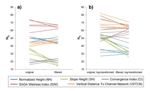
Fig. 7. Effects of (a) median filtering of DEMs and (b) log-transformation of land-surface parameters (LSPs) on the number of terrain segments that spatially correspond to drumlins ( $N_{Si}$ ). The higher the number, the better drumlin recovery through multiresolution segmentation (MRS). Results for five LSPs (color-coded).
