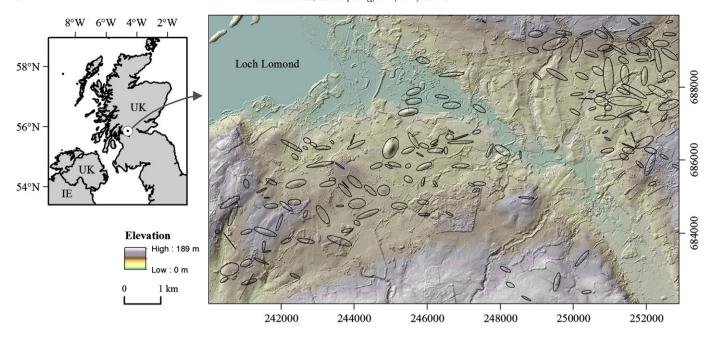
Fig. 1. Study area located in Scotland, UK. The large map illustrates the relief-shaded synthetic 5-m DEM 1 with superimposed outlines of the randomly placed synthetic drumlins (*n* = 173). The DEM is colored according to elevation. Map coordinates are British National Grid.
