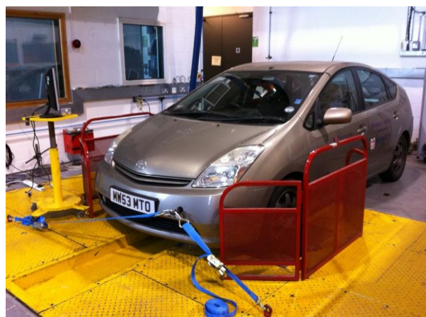
Figure 1: Toyota Prius test vehicle on chassis dynamometer.
