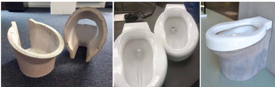
Figure 5. Final design provides full height, semi-squat & urinal design from one mould. Two piece GRP bowl/urinal & seat provide reduced shipping footprint
