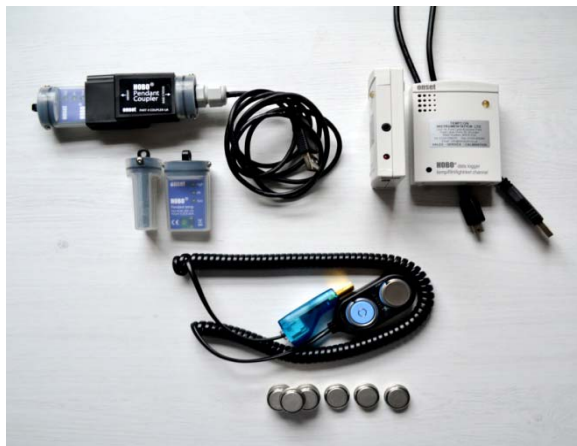
Figure 3 HOBO pendants for room air temperature, HOBO U12 for room air temperature, illuminance and humidity levels and 1-wire ibuttons for surface temperature monitoring.
