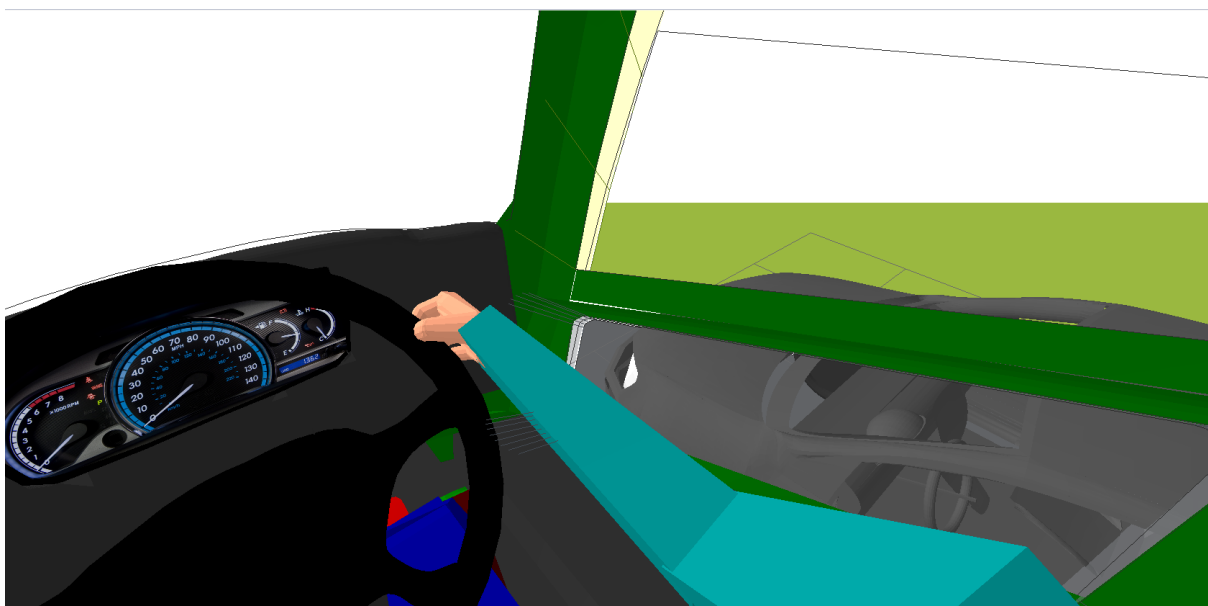
Figure 142. Driver's eye view. Plan view. The car can be seen by the driver of the category N 3 vehicle.
