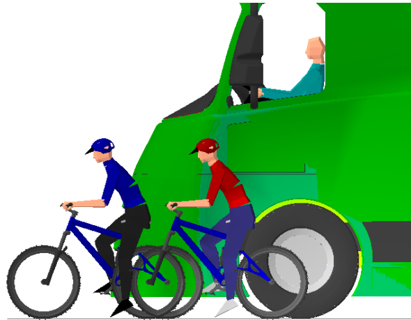
Figure 19. The configuration of the cyclist visual targets positioned to the offside of the vehicle
