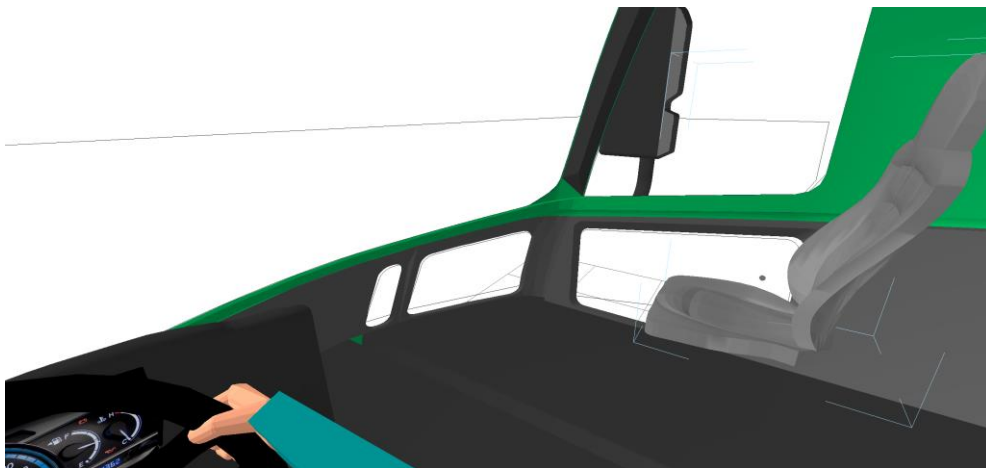
Figure 146. A passenger seat has the potential to reduce the effectiveness of the lower passenger door window
