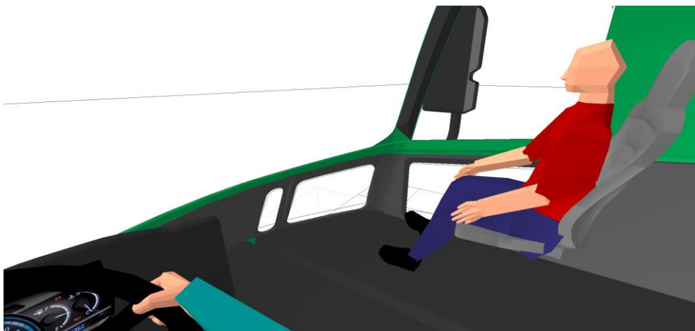
Figure 147. A passenger occupying the passenger seat has the potential to further reduce effectiveness of the lower passenger door window
