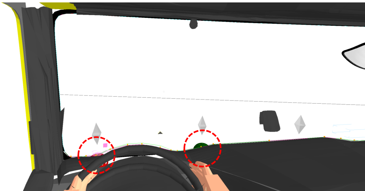
Figure 35. Driver's eye view. Small portions of the red and green cyclist helmets can be seen by the driver of the category N3 vehicle.
