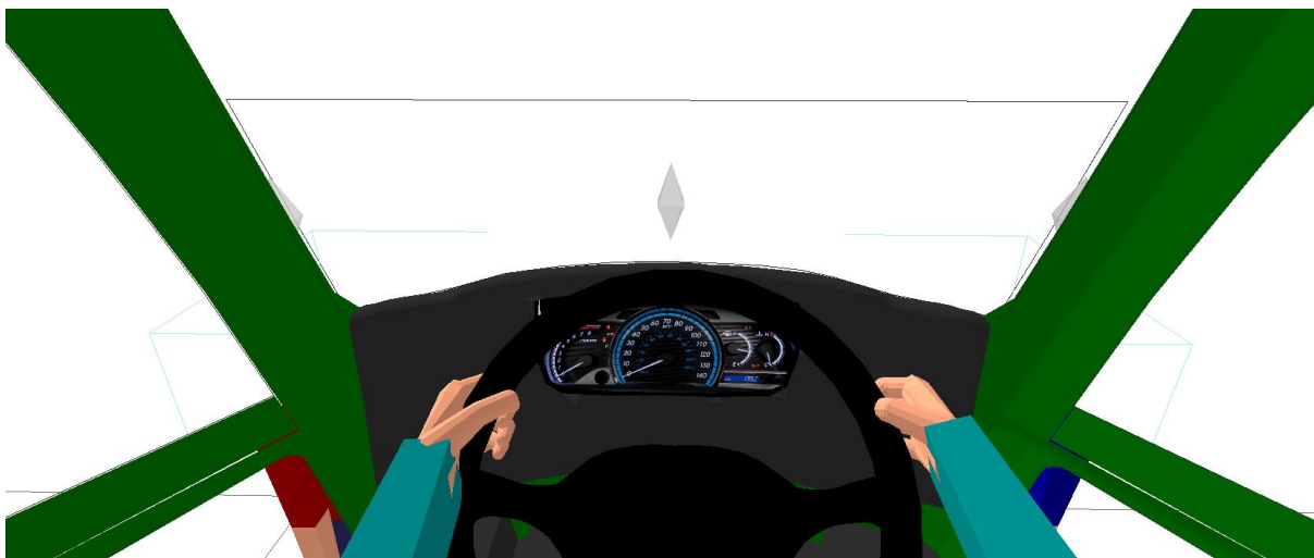
Figure 127. Driver's eye view. The red and blue pedestrians can be seen. The green pedestrian can be 97mm in front of the centre of the vehicle and not be seen due to obscuration by the dash structure
