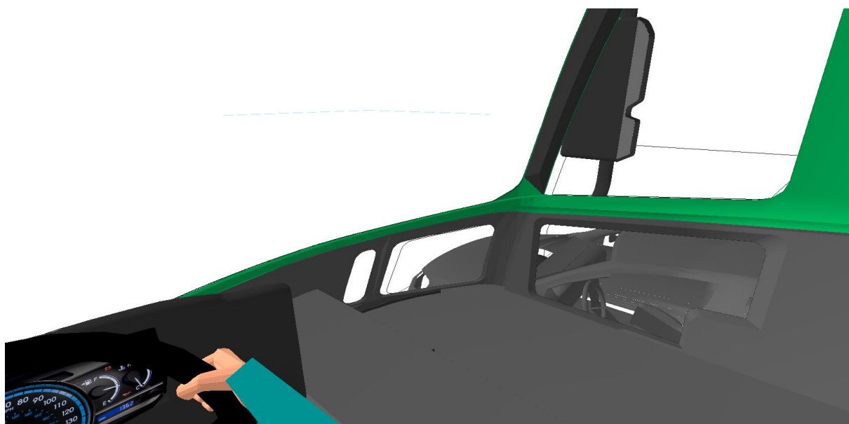
Figure 120. Driver's eye view. The car be seen by the driver of the category N3 vehicle through the lower window door and the right hand lower window
