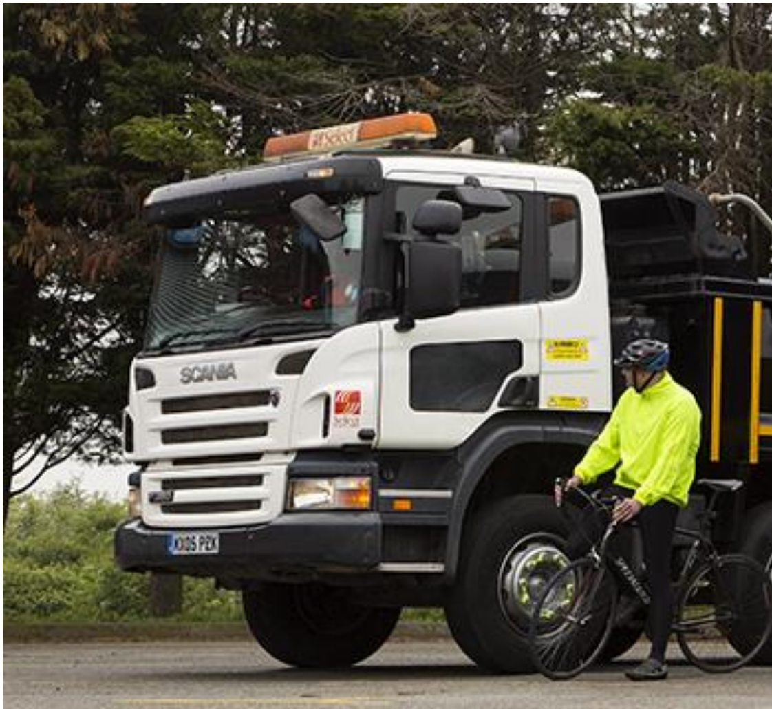
Figure 7. The additional side windows added to Scania Vehicles in collaboration with Laing O'Rourke
