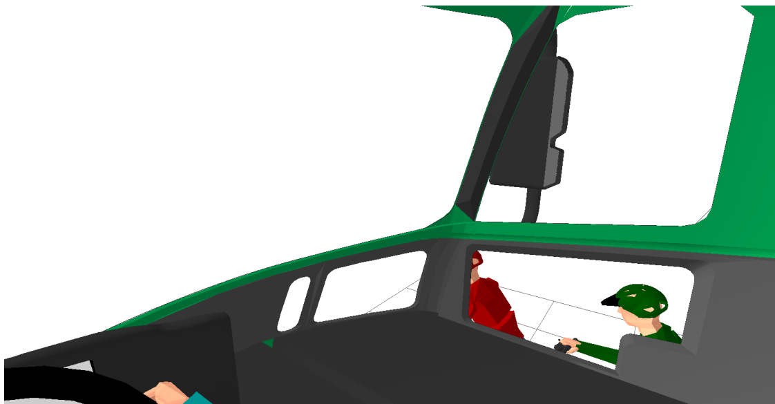
Figure 95. Driver's view of the cyclists positioned to the nearside of the vehicle, the rear (green) and front (red) cyclists are both clearly visible through the lower door windows
