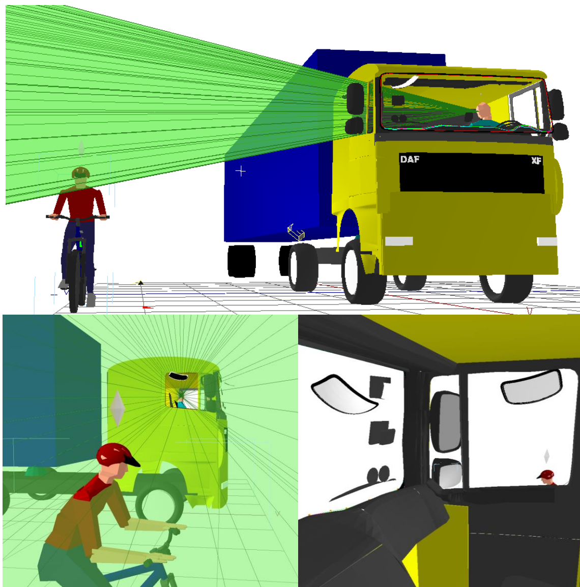
Figure 16. An illustration of the aperture projection technique used in the SAMMIE DHM system. The green semi-transparent volume represents the volume of space visible to the driver through the passenger window.
