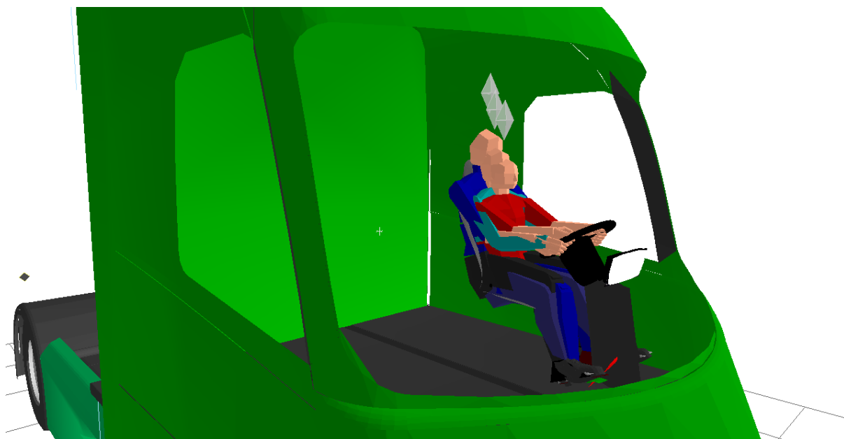
Figure 5. The occupant accommodation package from the DAF XF 105 placed within the FKA prototype.
