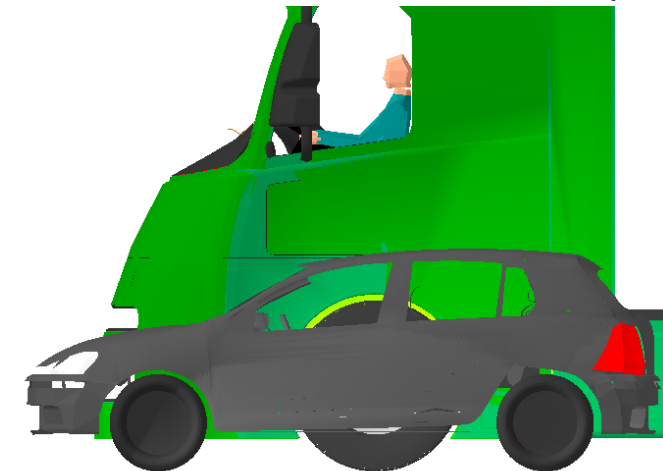
Figure 20. The configuration of the car visual target positioned to the offside of the vehicle
