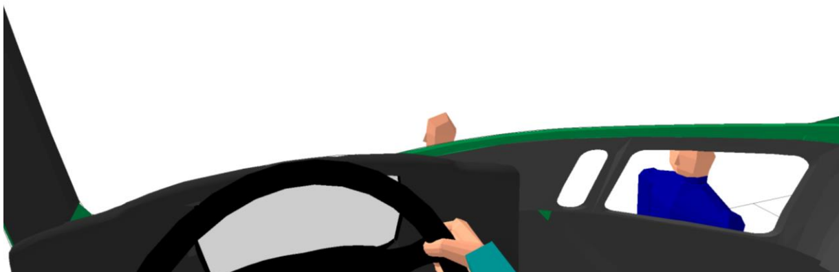
Figure 79. Driver's view of the pedestrians positioned to the front of the vehicle, the central (green) and right (blue) pedestrians are visible
