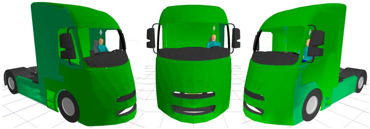
Figure 4. The FKA concept vehicle which takes advantage of additions to vehicle length by adding an aerodynamic nose section in front of the driver
