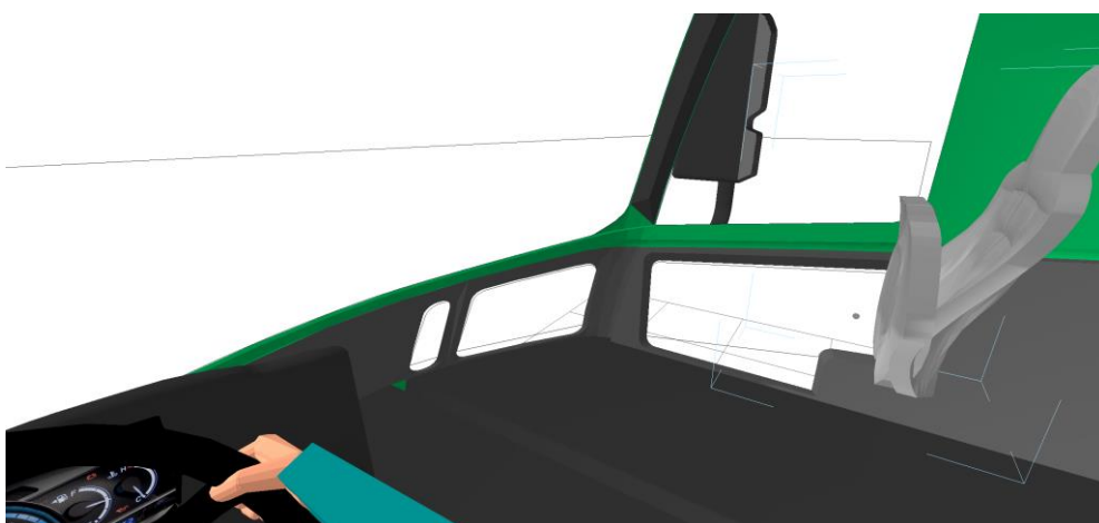
Figure 148. An unoccupied passenger seat can allow full view of the lower passenger door window if it is foldable
