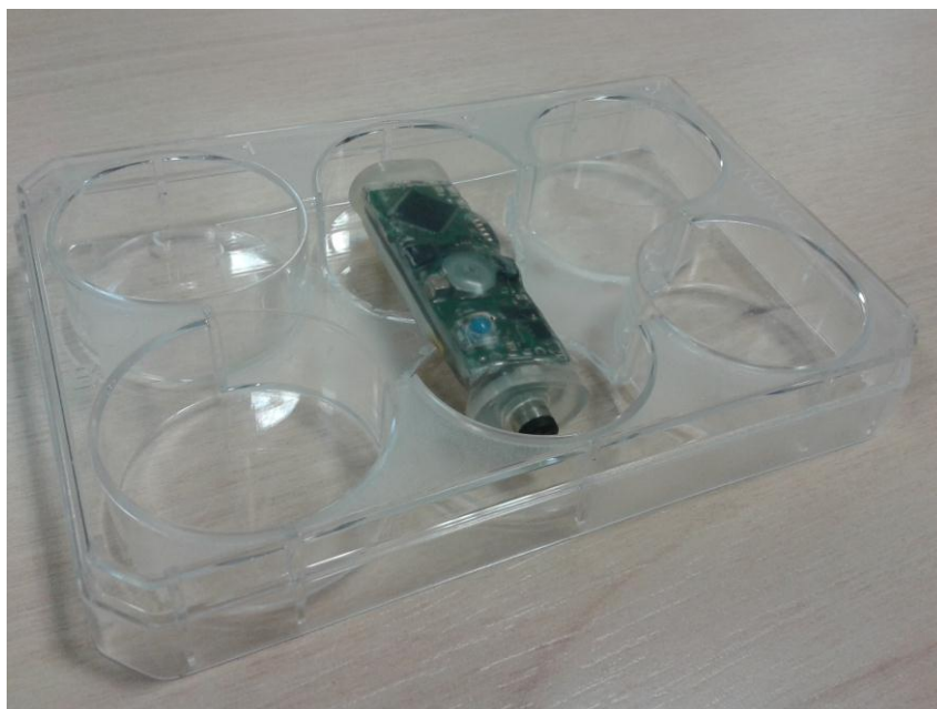
Figure 94. Adapted 6-well plate with humidity and temperature sensor MSR 145. By removing the central walls of wells A2 and B2 on a 6-well plate the sensor can fit in the centre whilst wells A1, B1 and A3, B3 can still be used for culture.
