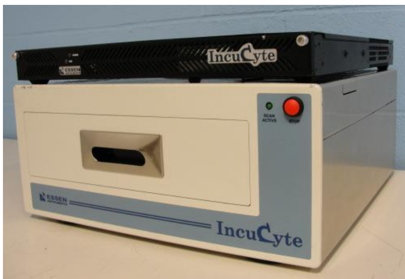
Figure 9. Essen Bioscience compact microscope, IncuCyte (69) The Incucyte system allows you to place a microscope within an incubator. With configurable trays a wide variety of culture vessels can be used within the system to provide long-term live cell imaging.
