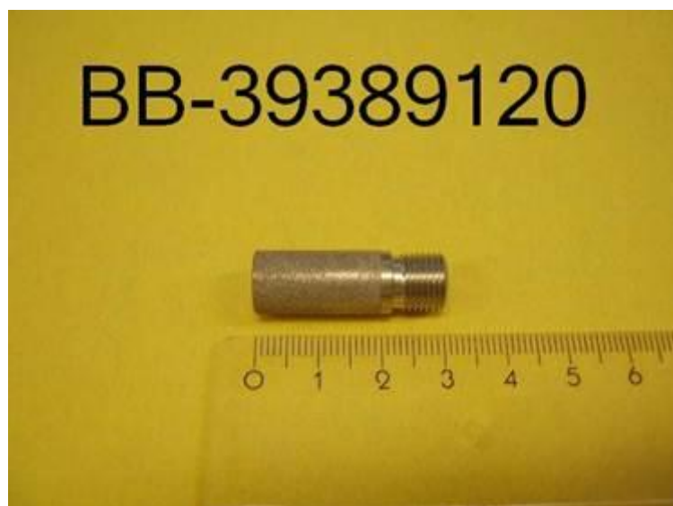
Figure 103. 20 \mu\text{m} fermentation sparger. Adapted from a fermentation bioreactor sparger, this Sartorius sintered metal sparger can be sterilised and used to increase the surface area of gas bubbles in contact with liquid, therefore improving humidification.
