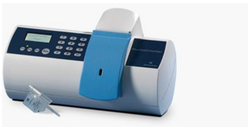
Figure 14. Chemometec NucleoCounter NC-100. A compact cell counter using pre-loaded propidium iodide cassettes to determine count and viability of a sample (80).
