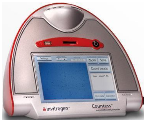
Figure 16. Life Technologies Countess, automated cell counter. The Countess uses prepared slides containing cell sample and trypan blue, then uses image analysis to measure viable and non-viable cells (82).
