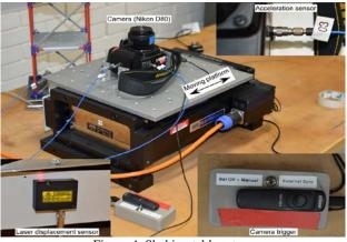
Figure 4. Shaking table setup.
