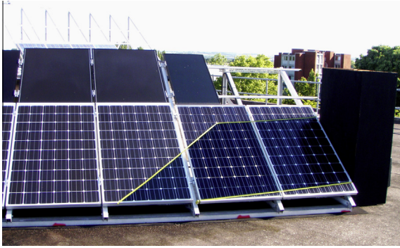
Fig. 14a. Scenario1, ‘Chimney’ to side of array with shadow marked out with yellow tape.
