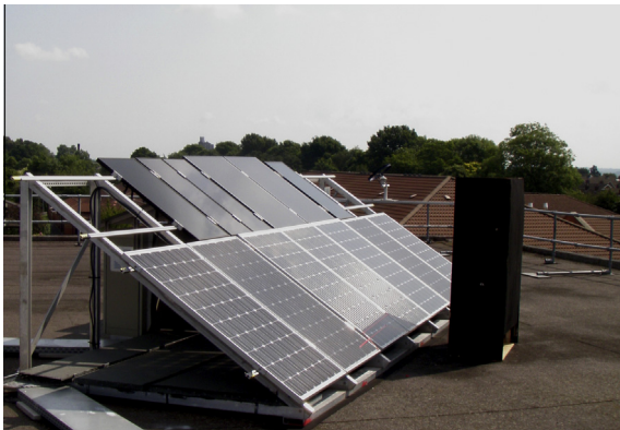
Fig. 14b. Scenario 2, ‘Chimney’ obstruction to front of array.
