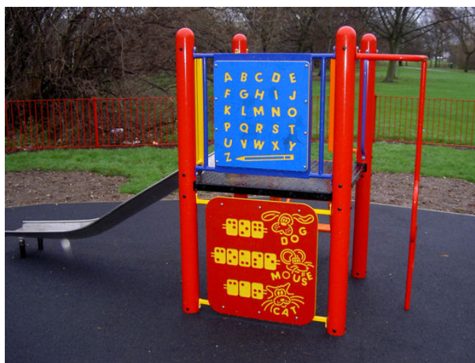
Figure 6: Multi-modal displays attached to a slide in a playground area in Loughborough, England. This example shows on one display, the letters of the alphabet as recessed characters which can be seen and detected by touch. The display below shows the images of three pet animals (dog, mouse, cat) with the names also presented as recessed letters and with Braille equivalent letters alongside.
