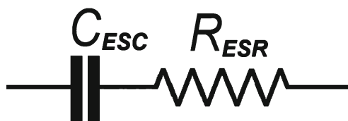
Fig. 1 An example of an engineering equivalent circuit. At each measurement frequency, the capacitance and resistance values are adjusted to match the amplitude and phase response of the real system. The resulting values of C and R are then referred to as “the equivalent series capacitance” (ESC) and “the equivalent series resistance” (ESR)
