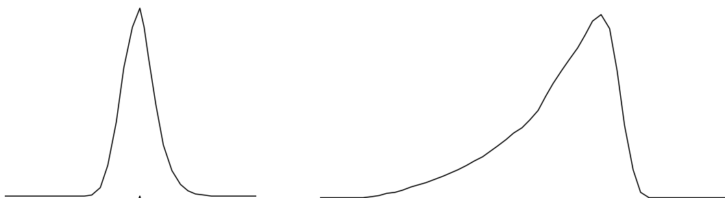
Figure 2.10 Extracted ion chromatograms for octanal ( m/z 56, left) and octanoic acid ( m/z 60, right) showing the different peak shapes obtained from VOC profiles using the methods applied in this thesis. Chromatographi peak shape is a key consideration in the development of automated data processing methods.
