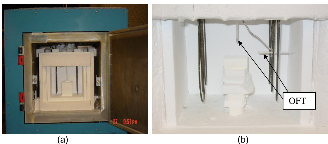
Figure 82 Hybrid furnace showing (a) front view and (b) furnace space with placement of the OFT (mode stirrer is obstructed by the alumina fibre insulation)
