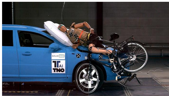
Figure 2.7 External airbag performing during crash test with pedestrian dummy on cycle (TNO, 2012)
