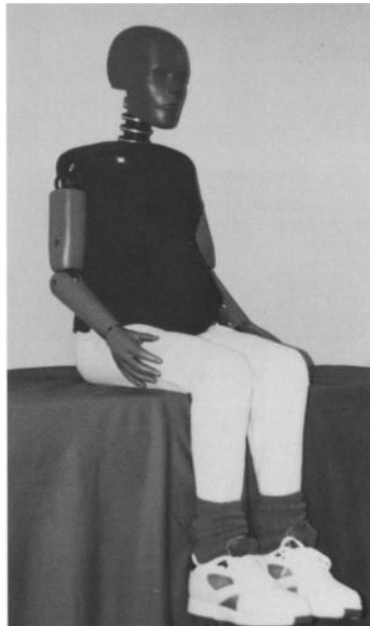
Figure 3.5 Urethane pregnancy insert and chest skin for the 5th percentile pregnant Hybrid III dummy (Pearlman et al. , 1996)
