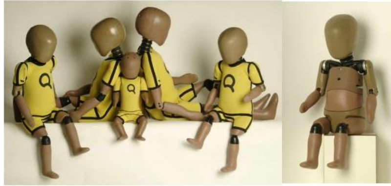
Figure 2.4 The Q series child dummy family :( from left to right) Q1.5, Q3, Q6, Q1 and Q1 without suit (Jager et al. , 2005)
