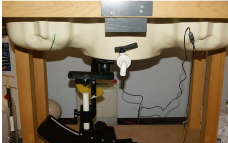
Figure 3-12: Smart phone positioned in the flat section of the twin phantom with HFK connected to the ear of the left head of the phantom
