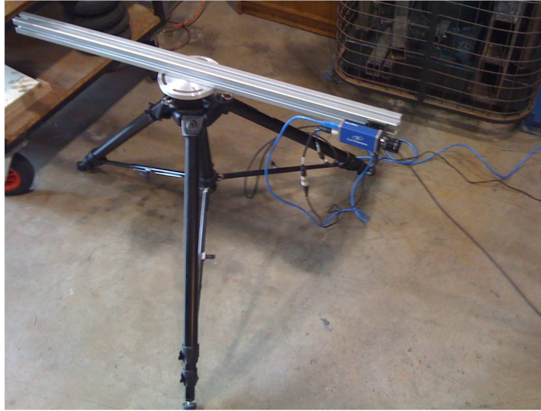
Figure 6.14: Position of the camera in the DIC experiment.
