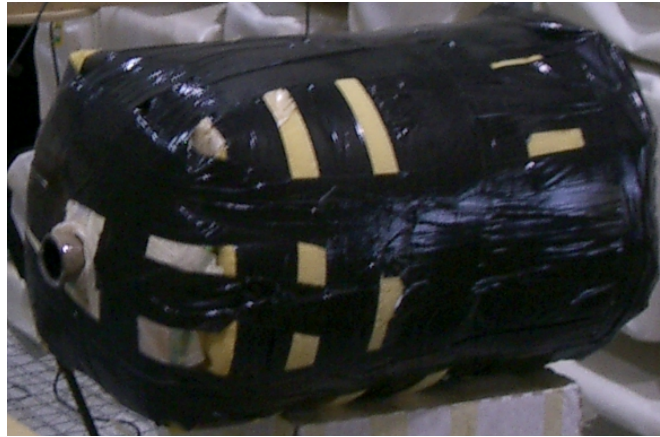
Figure 4.2: Photograph of the exhaust orifice noise source (orifice on the left).
