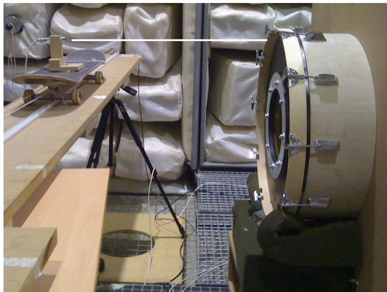
Figure 6.58: Photograph of the TSR test rig in the reciprocal arrangement of the laboratory scale pass-by noise experiment. The pass-by noise microphone and the top of the sidewall are on the same height.
