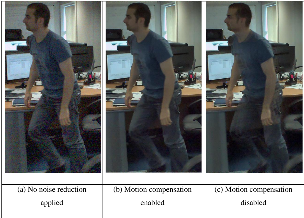
Figure 20: Experimental results, Motion Compensation evaluation.
