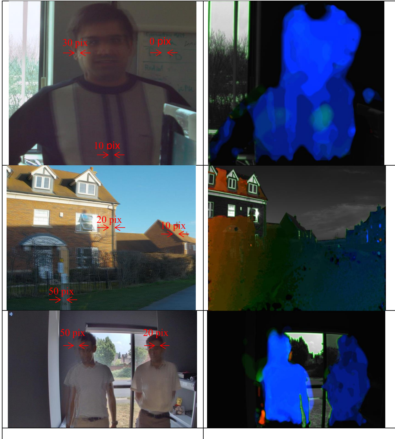
Figure 36: Example of motion and calculated motion field.
