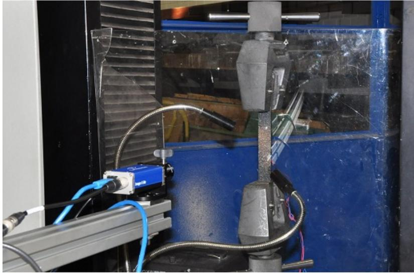
Figure 5: Experimental set-up for tensile tests with a DIC system.
