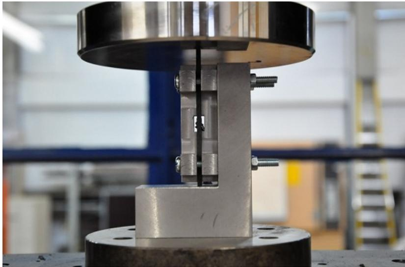
Figure 6: Experimental set-up for compression modulus tests.
