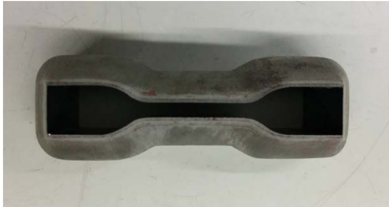
Figure 7: Dogbone specimen sample stamp (cutting edge) - 80mm long, 25x4mm gauge length
