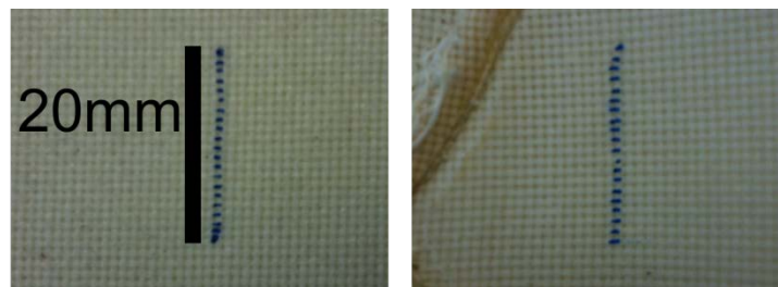
Figure 27: Carcass fabric before assembly (left), and cut from an assembled ball (right)
