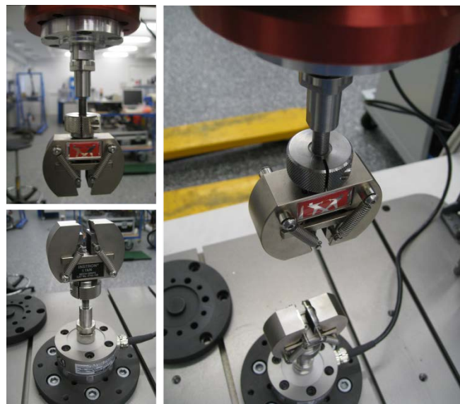
Figure 12: ElectroPuls, lightweight clamps, base-mounted load cell
