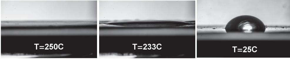
FIGURE 2.4: Shown is from right to left a series of experimental images showing the change of the contact angle of water on sapphire (complete wetting to almost non-wetting case). Reproduced with permission of the authors from [40].
