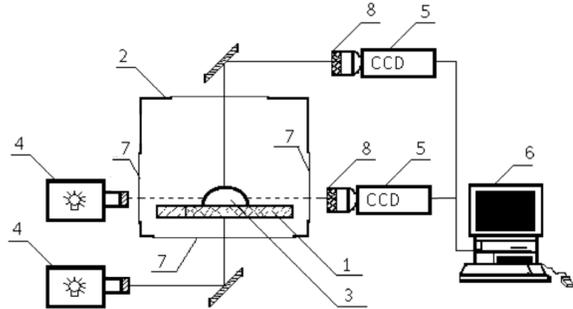
Fig. 1. Sketch of the experimental set-up: 1, porous substrate; 2, hermetically closed, thermostated chamber; 3, liquid drop; 4, light sources; 5, CCD cameras; 6, PC; 7, optical windows; 8, optical objectives.
