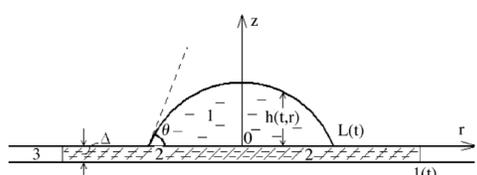
Fig. 2. Cross-section of the axis-symmetric spreading drop over initially dry filter paper with thickness  $\Delta$ . 1 - liquid drop; 2 - wetted region inside the porous substrate; 3 - dry region inside the porous substrate.  $L(t)$  - radius of the drop base;  $l(t)$  - radius of the wetted area inside the porous substrate;  $\Delta$  - thickness of porous substrate,  $r, z$  - coordinate system;  $h(t, r)$  - profile of the spreading drop;  $\theta$  - contact angle.
