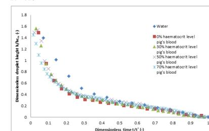
Fig. 8. Dimensionless droplet heights of water, blood 0%, 30%, 50% and 70% haematocrit blood as function of dimensionless time
