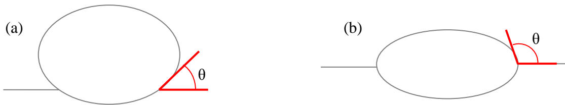
Figure 11: Schematic of wetting angles ( \theta ) showing (a) acute wetting angle, giving poor clad track (b) obtuse wetting angle, giving successful clad track
