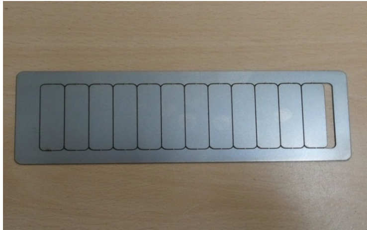
Figure 6: Sample plate with twelve individual sample coupons
