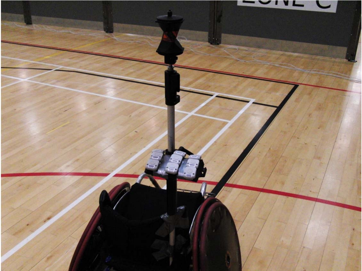
Figure 4: Tags and prism mounted on a wheelchair
