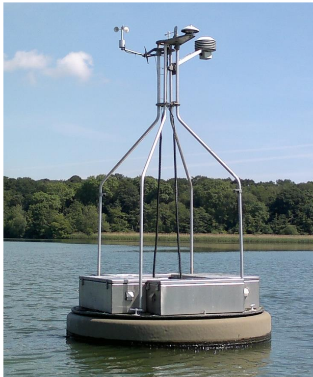
Figure 2.8 Automatic weather and water quality monitoring station on Rostherne Mere, Cheshire.
