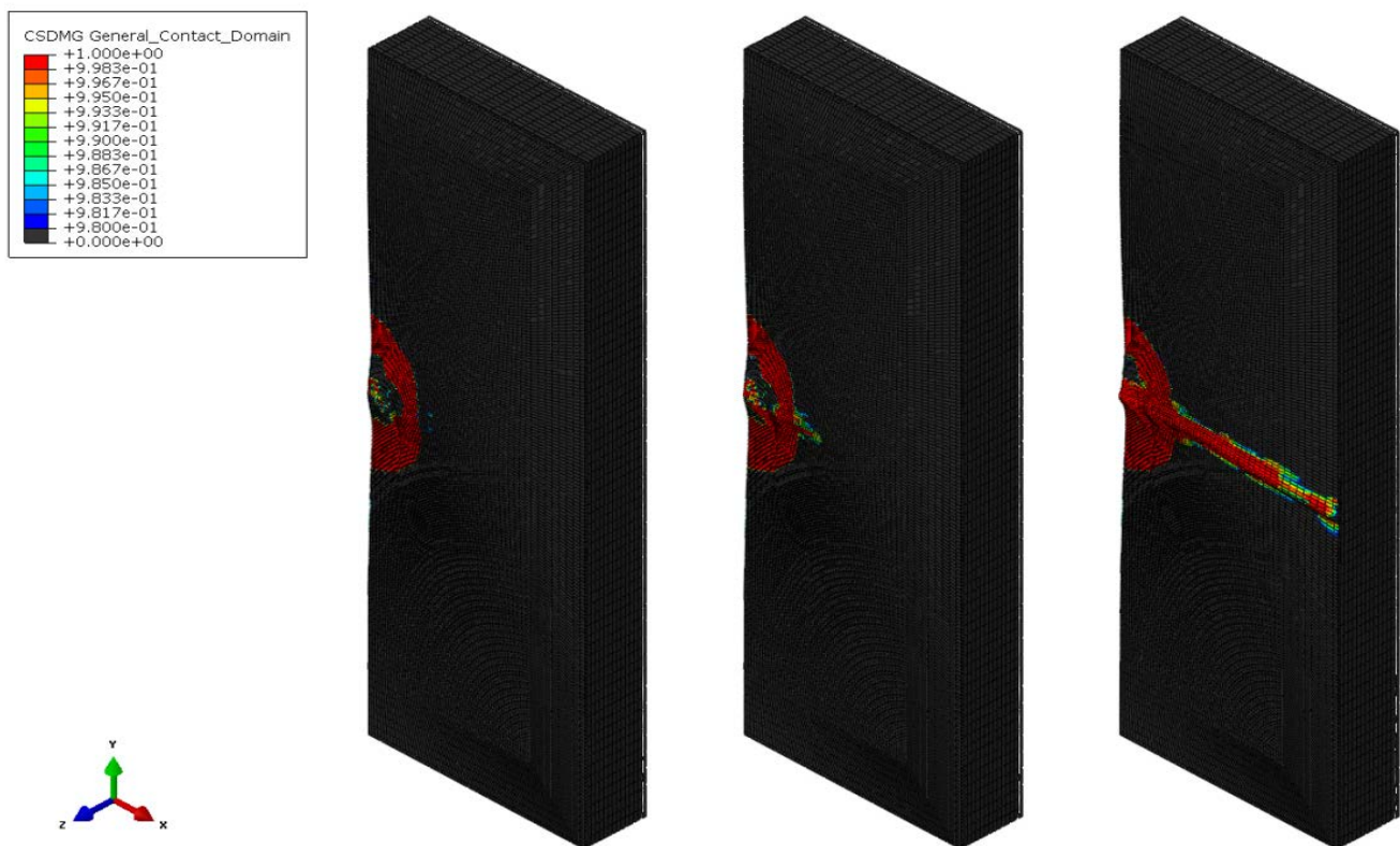
Figure 10. Delamination propagation in S7 . The leftmost frame shows the panel just prior to final failure, with the delamination growing outwards from the damaged region to the fully-developed state in the rightmost frame. The delamination propagated to full-width in less than 0.2ms.
