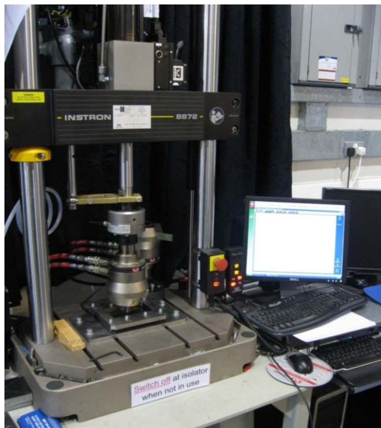
Figure 2. Indentation fixture within Instron 8872 machine
