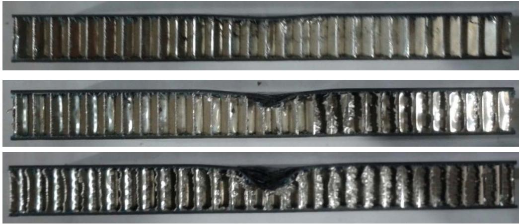
Figure 3. Sectioned symmetric panels after quasi-static-indentation with (from top) a) 2.5mm, b) 5mm, c) 7mm applied displacement. Note the ‘cup’ of damaged fibres in (c) which is approximately the same diameter as the indenter – 16mm.
