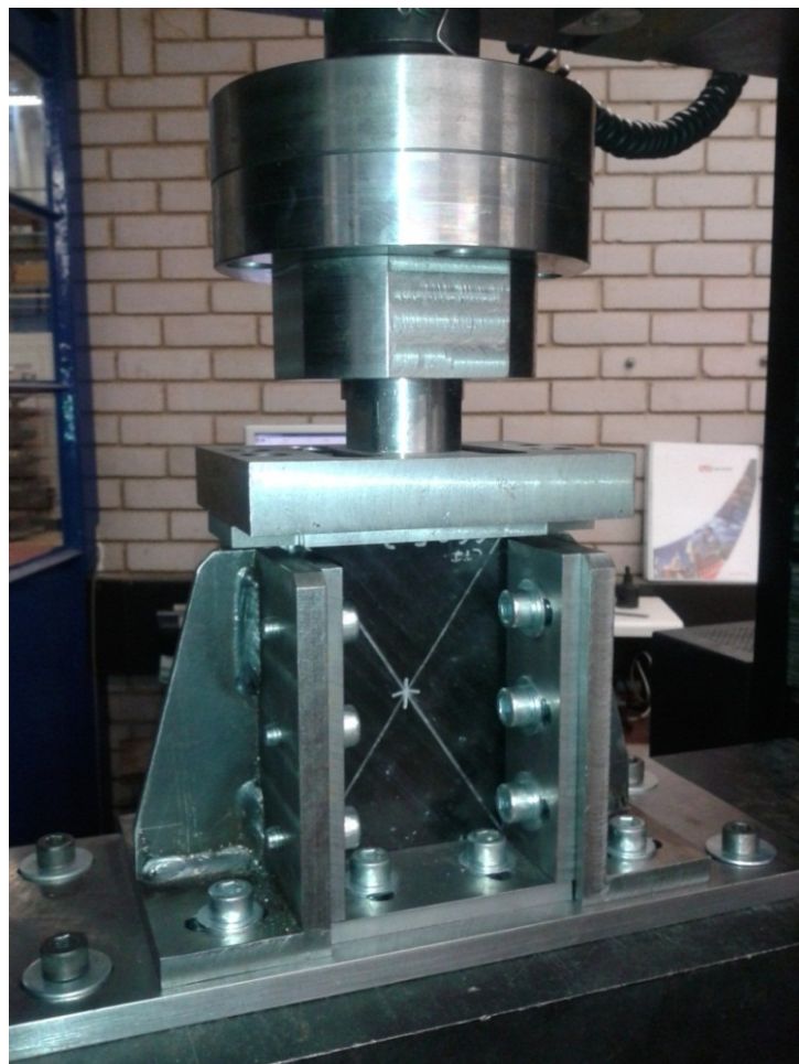
Figure 1. A panel loaded into the compression-after-impact fixture, ready for testing
