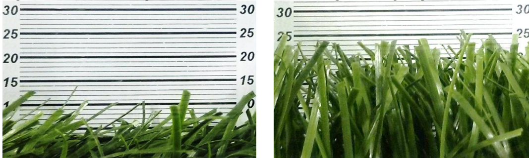
Figure 1 - Free pile height photos from different areas of the same pitch. Photo on the left from location E and photo on the right from location F. The twenty tallest fibres in each photo are averaged to calculate the free pile height measurement.
