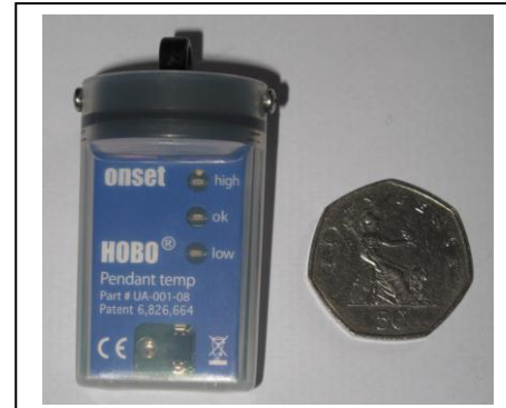
Figure 2. Hobo data logger used to measure indoor air temperature.
