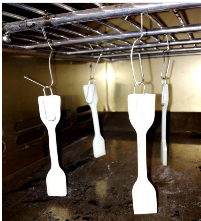
Fig. 3.13: Aged test sample in a cell-type oven with no strain
