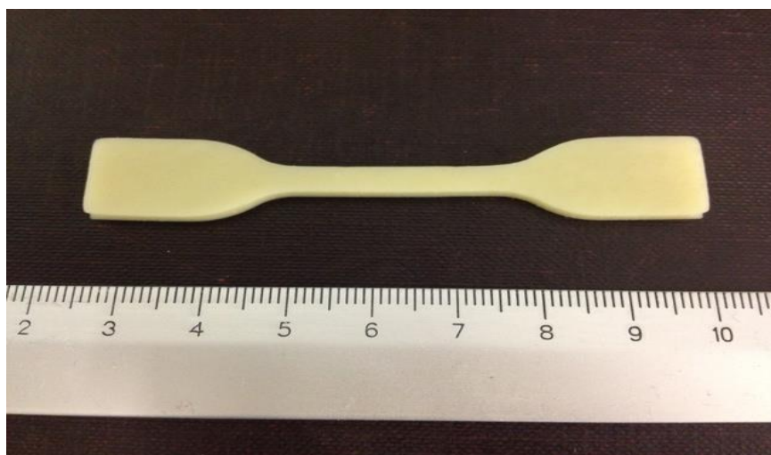
Fig. 3.8: Dumbbell test pieces Type 1 [Test length: 25 \pm 0.5 mm]
