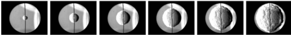
Fig.4-5. Experimental images in the sequence of propagation. Measured flame radiuses are: 5.8, 12.1, 17.8, 23.9, 30.0 and 35.0mm. H 2 -Air mixture at 298K, 1bar and \Phi=0.6 .
