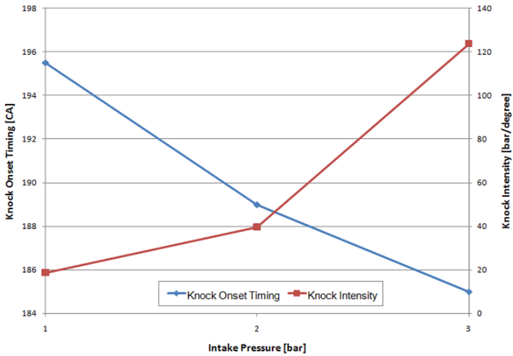
Fig. 6-6 Calculated knock onset timing and intensity at different intake pressures. Other initial conditions are 1500RPM, 373K, \phi=1.0 and ignition at 9°BTDC.
