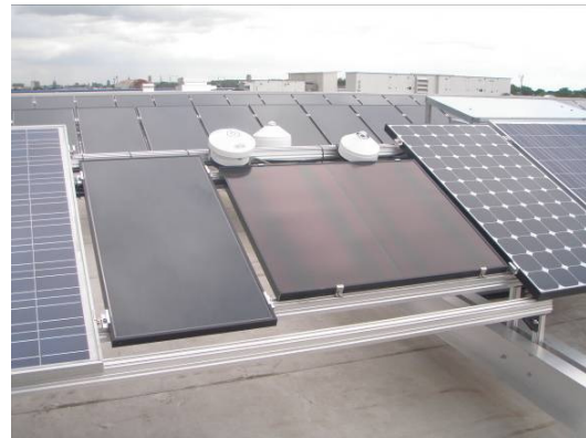
Figure 2: Sensors measuring horizontal and plane-of-array irradiance and spectral distribution.
