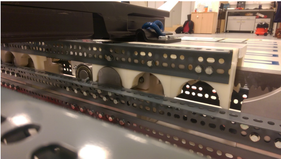
Figure 9: Close up photograph of actuation cam and locking block protrusions
