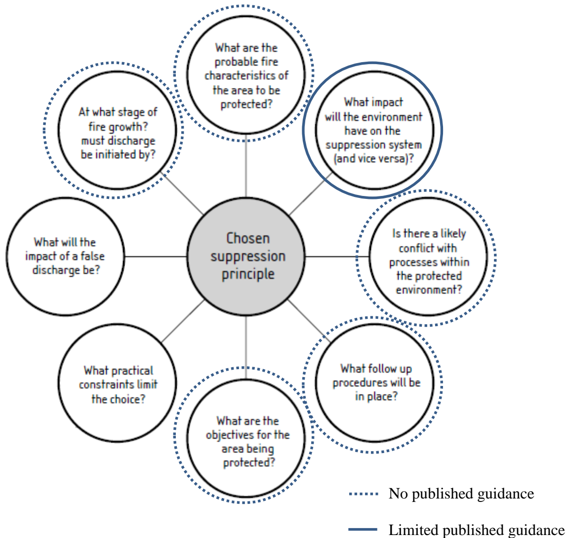
Figure 2.1: Fire suppression system choice matrix (adapted from (BSI, 2003c)).
