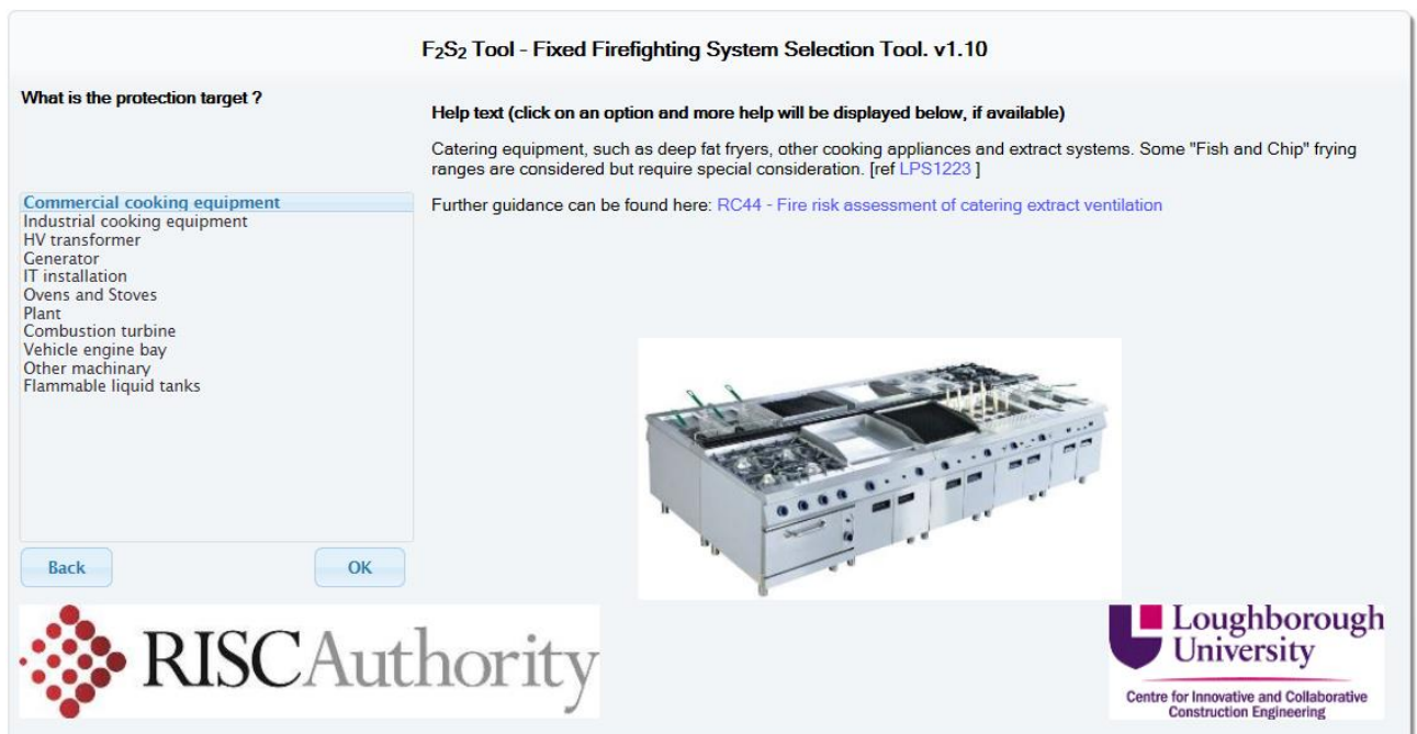
Figure 4 - Example of Graphical User Interface (GUI) – displaying ‘object’ protection scenarios and help text and graphic for ‘Commercial cooking equipment’
