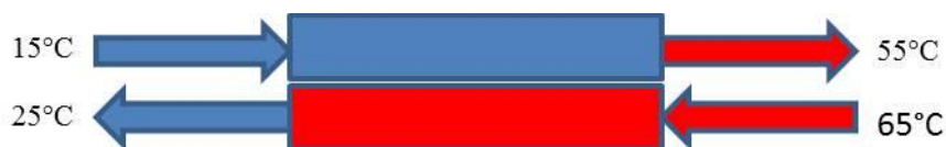
Figure 4- 18 Cross flow heat exchanger for \dot{m}_1 = \dot{m}_2 and with inlet temperatures of 65°C and 15 °C.
